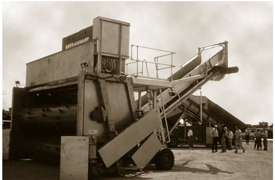
Figure 3. Pre-wet mixing machine.
